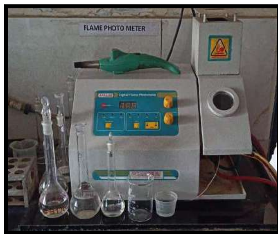
Analysis of Sodium, Calcium, Magnesium etc. by flame photometer
